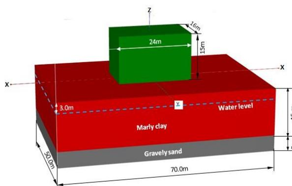
**Figure 1:** 3D Geometric model established by PLAXIS<sup>3D</sup> code
