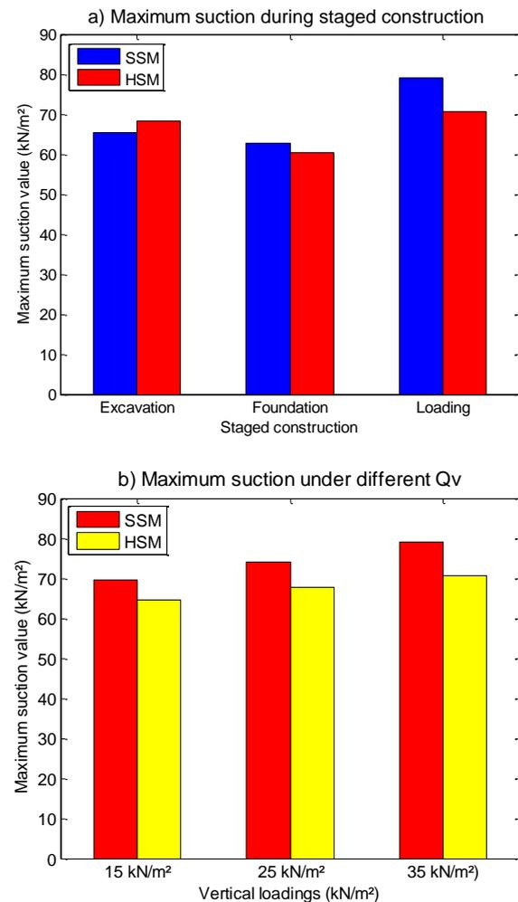
**Figure 6:** Maximum soil suction values during the project achievement and under different vertical loading  $Q_v$  values
