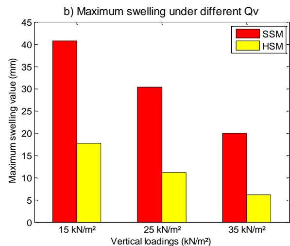
**Figure 4:** Maximum swelling values during the project achievement and under different vertical loading  $Q_v$  values
