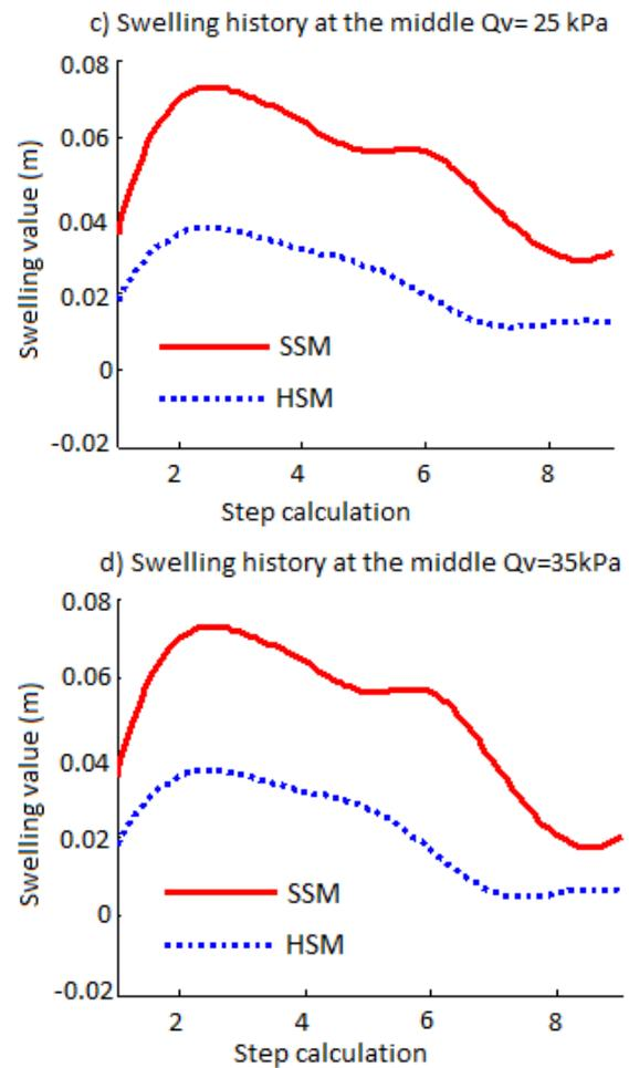
**Figure 7:** Swelling curve histories at the middle of the raft foundation during the construction period under different  $Q_v$  values
