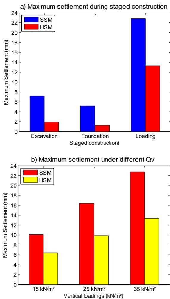
**Figure 5:** Maximum settlement values during the project achievement and under different vertical loading  $Q_v$  value
