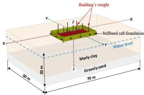
**Figure 3:** 3D equivalent model used in finite element analysis
