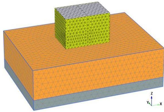
**Figure 2:** 3D finite element model mesh generated by PLAXIS<sup>3D</sup> code
