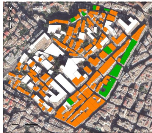
Figure 4: Strengthened masonry buildings classification map
